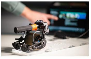
Composite testing: inspection results are displayed on the tablet screen. Any Windowsbased device can be connected to Krautkrämer RotoArray comPAct.
