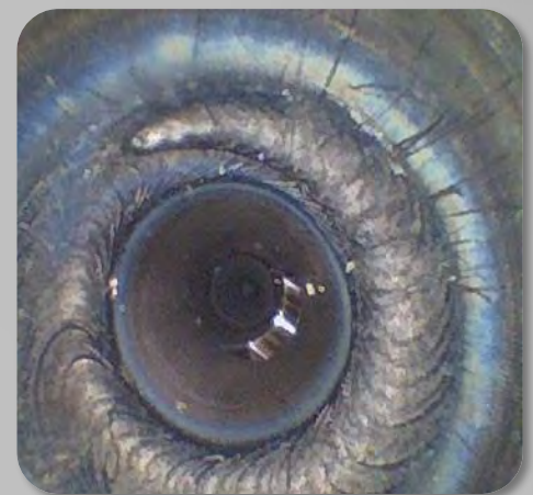
Stainless 1/3" Tube Orbital Weld Inspection using a .95mm VQ2 009 1000 NA
