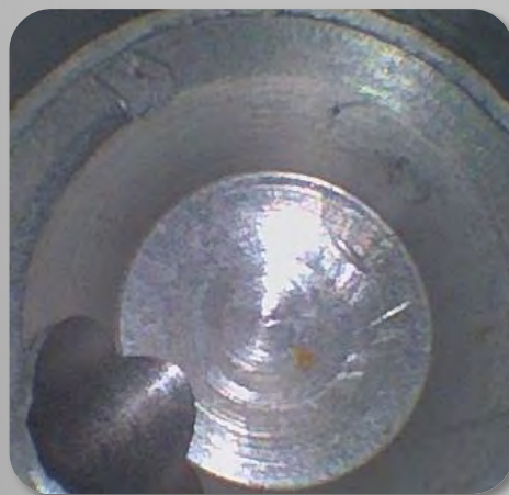
Metal Machined Cross Hole Inspection Using a 1.8mm VQ2 018 1000 NA
