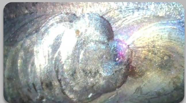
Orbital Weld Inspection Using a 4.5mm VQ2 045 1500 4D (Side View)
